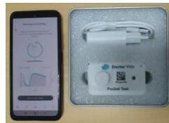
SmartLAMP SPOT is a smartphone-operated molecular diagnostic device using Loop-Mediated Isothermal Amplification (LAMP) to detect three key sweetpotato viruses: SPCSV, SPFMV, and SPLCV. It delivers laboratory-grade accuracy (100% agreement with Genie III) without requiring lab infrastructure, skilled personnel, or electricity. Each test takes ~40 minutes and can be performed on-site using a power bank.
